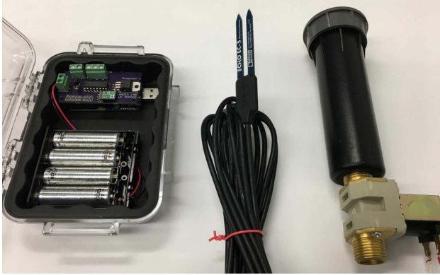
Figure 9: Sensing and actuation node
