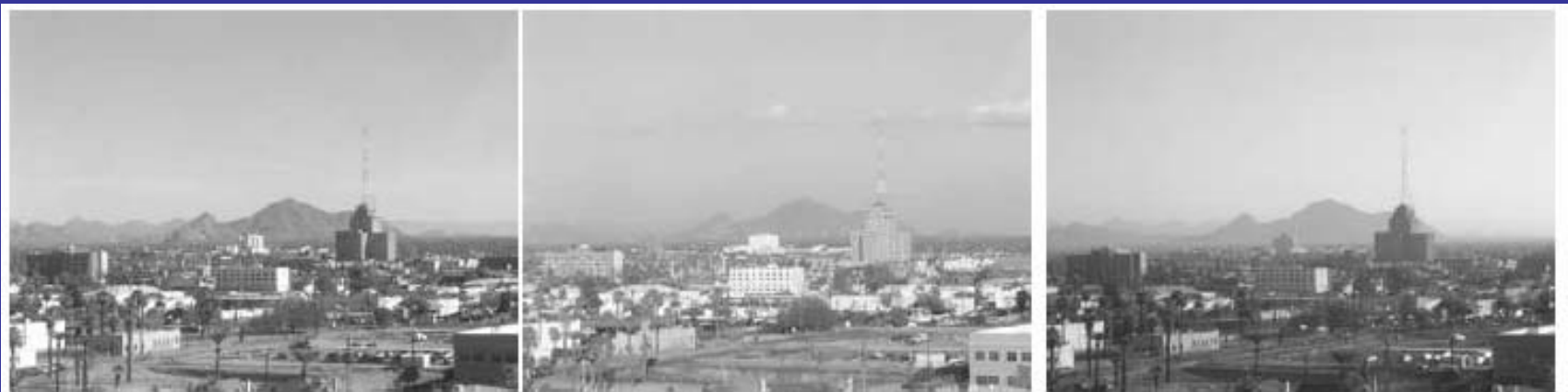
(a) b_{ext} = 9 \text{ Mm}^{-1} (b) b_{ext} = 28 \text{ Mm}^{-1} (c) b_{ext} = 163 \text{ Mm}^{-1}
