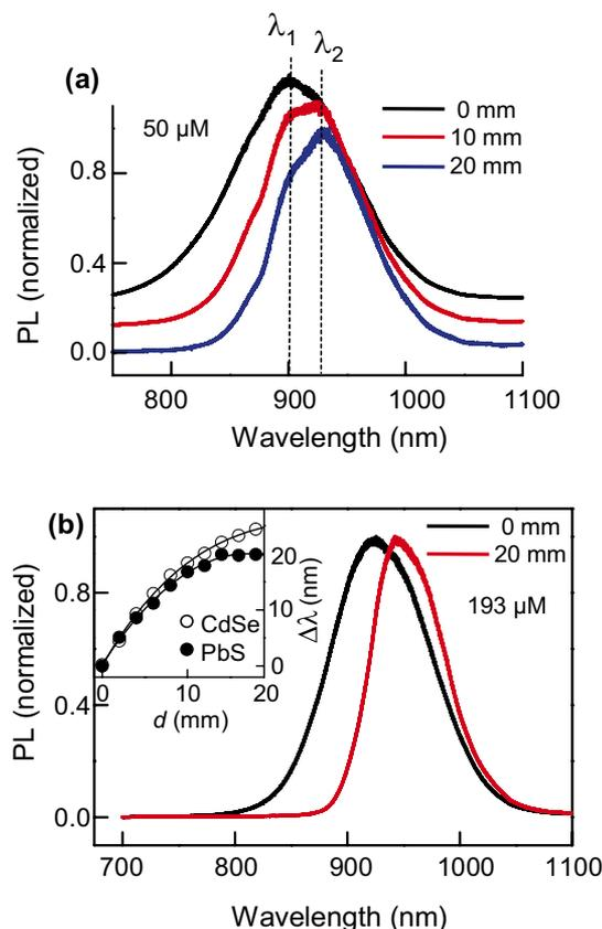
FIG. 2. (Color online) (a) The effect of changing the distance between excitation and collection points for a 50  $\mu\text{M}$  PbS sample on the emission spectrum. The graphs are shifted vertically for clarity. (b) Similar effect for a 193  $\mu\text{M}$  PbS sample. The inset compares the peak emission redshifts with distance for PbS and CdSe/ZnS samples.
