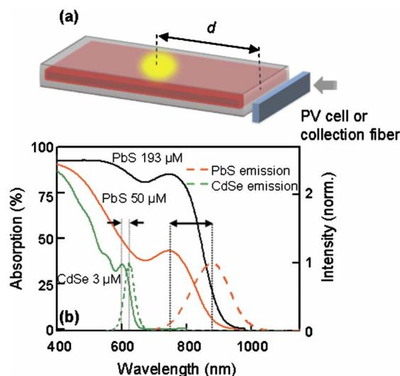
FIG. 1. (Color online) (a) Schematic of the device highlighting the arrangement of PV cell/collection fiber with relation to the excitation beam. (b) Absorption curves in absolute units for CdSe/ZnS and PbS QDs. Overlaid emission curves (dashed) for CdSe/ZnS and PbS QDs with Stoke's shift marked by double headed arrows.
