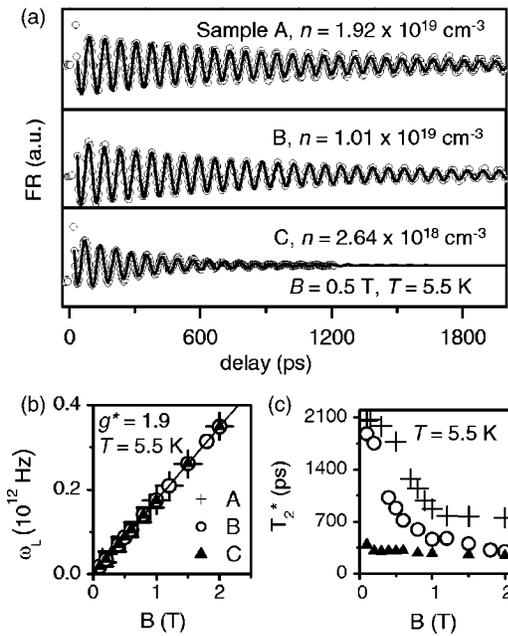
FIG. 1. (a) TRFR as a function of pump-probe delay for the Samples A–C at  $T = 5.5 \text{ K}$  and  $B = 0.5 \text{ T}$ . The carrier densities are indicated in the figure. Lines are fits using Eq. (1). (b) Larmor frequency  $\omega_L$  as a function of  $B$ . Line is a linear fit. (c) Spin coherence time  $T_2^*$  as a function of  $B$  at  $T = 5.5 \text{ K}$  for the same samples. The symbols in (c) correspond to those in (b).
