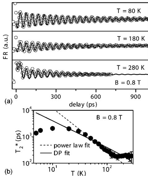
FIG. 2. Temperature dependence of TRFR on Sample A. (a) Spin precession at three temperatures for  $B = 0.8 \text{ T}$ . (b)  $T_2^*$  follows a power law (dashed line) with temperature in the intermediate region of 30 to 150 K, with an exponent  $-1.54 \pm 0.03$ . Theoretical fit to the data for DP mechanism is shown as a solid line.
