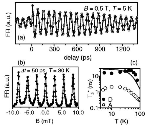
FIG. 3. (a) TRFR at  $T = 5 \text{ K}$  for the bulk Sample D. Line is a guide for the eyes. (b) Faraday rotation versus  $B$  at  $T = 30 \text{ K}$  and  $\Delta t = 50 \text{ ps}$  on Sample D showing multiple RSA peaks. Lines are Lorentzian fits. (c)  $T_2^*$  obtained from RSA peak at  $B = 0 \text{ T}$ , as a function of temperature for Sample D (filled circles) with results from Sample A (open circles) shown for comparison. The line is a theoretical fit of the DP mechanism for Sample D.
