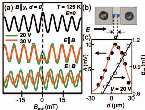
FIG. 2. (Color) Data from 100 nm sample at  $T=125$  K. (a) Kerr rotation with pump-probe overlapped ( $d=0$ ) at  $\Delta t=13$  ns with (top)  $E=0$ , (center)  $E\parallel B_{\text{ext}}$ , and (bottom)  $E\perp B_{\text{ext}}$ . (b) Schematic of measurement geometry for spatially resolved scans. (c)  $A$  and  $B_{\text{int}}$ , obtained from fits described in the text, as a function of pump-probe separation  $d$  with  $E\parallel B_{\text{ext}}$ .
