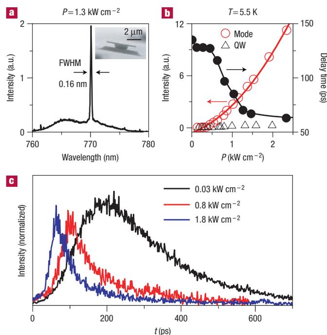
**Figure 1** Static and dynamical characteristics of microdiscs.
