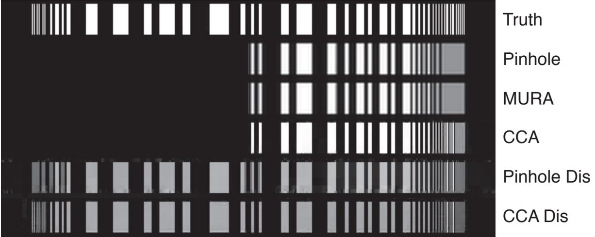
Figure 6. A comparison of the ground truth with the reconstructions using the five different setups: pinhole camera, camera with MURA coded aperture, camera with compressive coded aperture (CCA), disambiguation with a pinhole camera, and disambiguation with a camera using CCA. All five setups use the same FPA size. The pinhole, MURA, and CCA must be cropped, whereas the pinhole and CCA disambiguation setups superimpose the two halves onto the same FPA.
