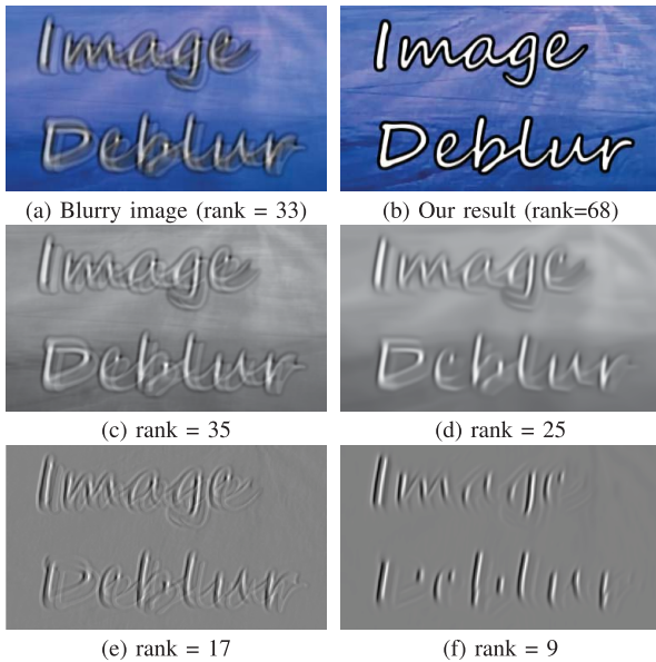
Fig. 1. The proposed low rank prior favors clear intermediate results which helps kernel estimation. (a) A blurry input. (b) Final deblurred image by the proposed algorithm. (c) Intensity map of (a). (d) Result by applying the proposed low rank model (2) on (c) without kernel estimation. (e) Gradient map of (a). (f) Result by applying the proposed low rank model (2) on (e) without kernel estimation.
