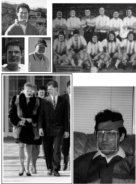
Figure 5.7: Sample experimental results using mixture of factor analyzers on images from three test sets. Every detected face is shown with an enclosing window.
