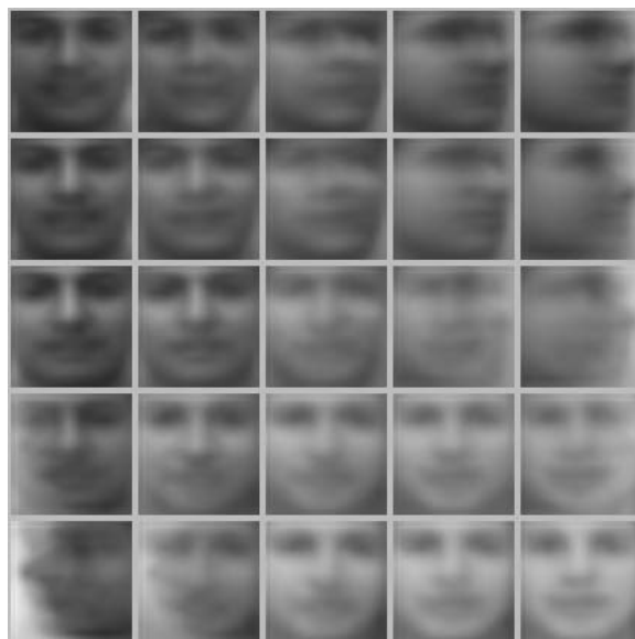
Figure 2.5: Prototype of each face class using Kohonen's SOM by Yang, Ahuja and Kriegman. Each prototype corresponds to the center of a cluster.
