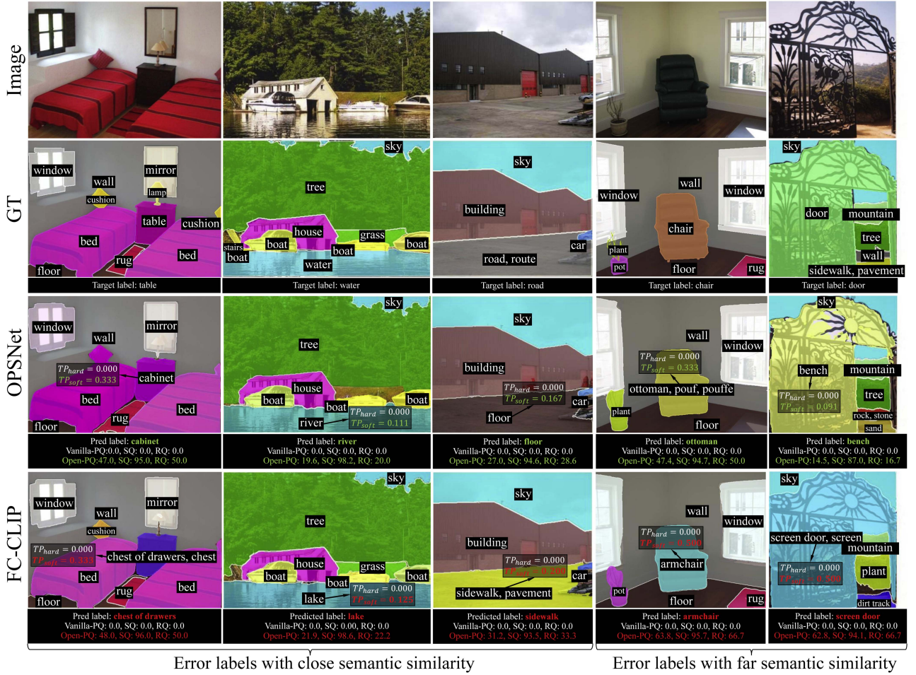
Fig. 1. Segmentation results with error labels evaluated by vanilla and open metrics. Our open metric assigns soft true positive (TP) for entities with error labels and thus provides a more reasonable evaluation for open-vocabulary segmentation.
