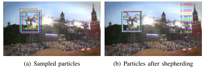
Fig. 2. A multi-task correlation filter is used to shepherd the sampled particles toward the modes of the target state distribution. The numbers in (b) are the scores of the correlation filter for the particles. Different colored boxes indicate the respective locations and scores.
