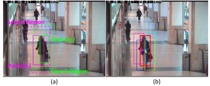
Fig. 4. The MCPF can cover object state space well with a few particles. Each particle corresponds to an image region enclosed by a bounding box. (a) The MCPF can cover object state space well by using a few particles with the search region where each particle covers the state subspace corresponding to all shifted region of the target object. (b) The MCPF can shepherd the sampled particles toward the modes of the target state distribution, which correspond to the target locations in the image.
