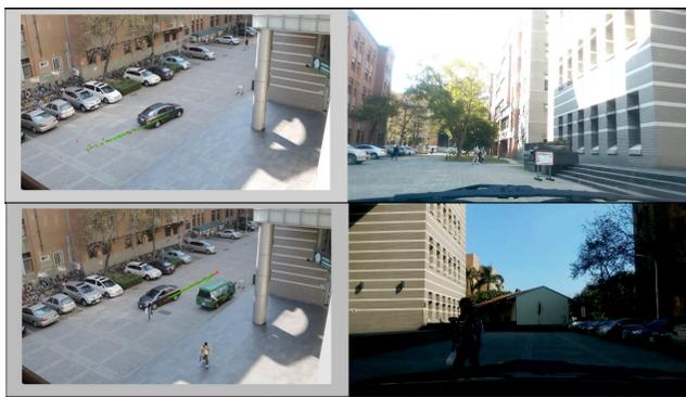
Fig. 13. Evaluation results using image sequences. Right column: an image from a dash camera. Left column: an image from a camera on third floor where red and green circles are the positioning results with still images and the results after temporal smoothing by the Kalman filter.
