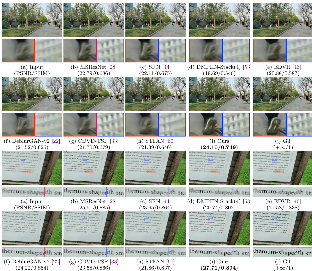
Fig. 9 Quantitative evaluations on our 4K resolution deblurring datasets. Our UHDVD generates much clearer images with higher PSNR and SSIM (zoom in for best view)
