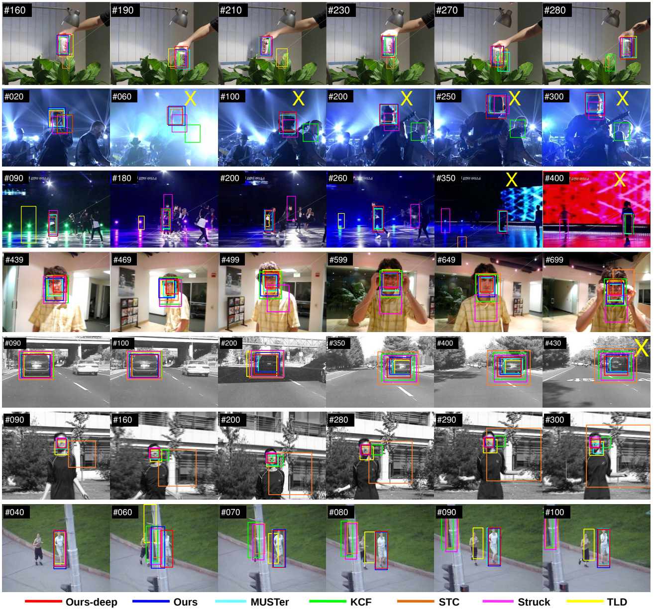
Fig. 16 Qualitative comparison. Tracking results on the seven challenging sequences are from our approach, the MUSTer [26], KCF [24], STC [55], Struck [21] and TLD [28] algorithms ( \times : no tracking output). The proposed method performs favorably against the baseline trackers in terms of both translation estimation and scale estimation. From first to last row: coke , shaking , skating1 , david , car4 , jumping and jogging-2 .
