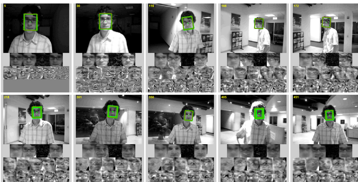
Figure 6: A person moves from a dark to a bright area, undergoing large lighting and pose changes. The images in the second row show the current sample mean, tracked region, reconstructed image, and the reconstruction error respectively. The third and fourth rows show the top 10 principal eigenvectors.
