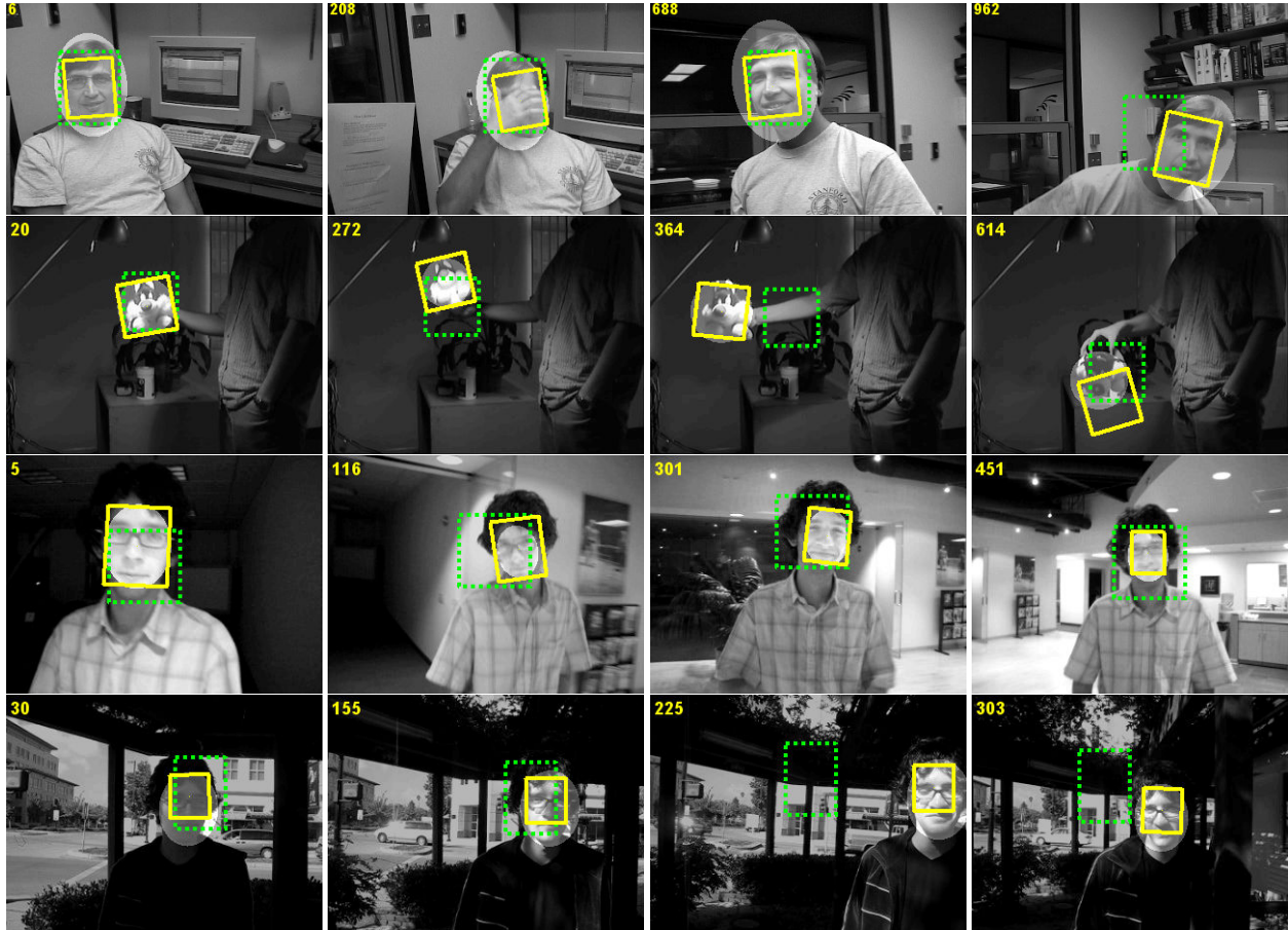
Figure 10: A comparison of our tracker (indicated with a yellow box) with the WSL [17] (shown in highlighted ellipse) and the Mean Shift [8] (depicted by a green dashed box) on four video sequences.
