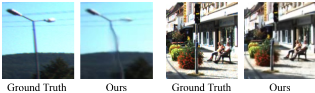
Figure 7: Failure cases. Due to the extremely narrow geometries (e.g., street light pole) and inhomogeneous diffuse reflections, our method fails in modeling these areas and generates images distorted and misaligned.
