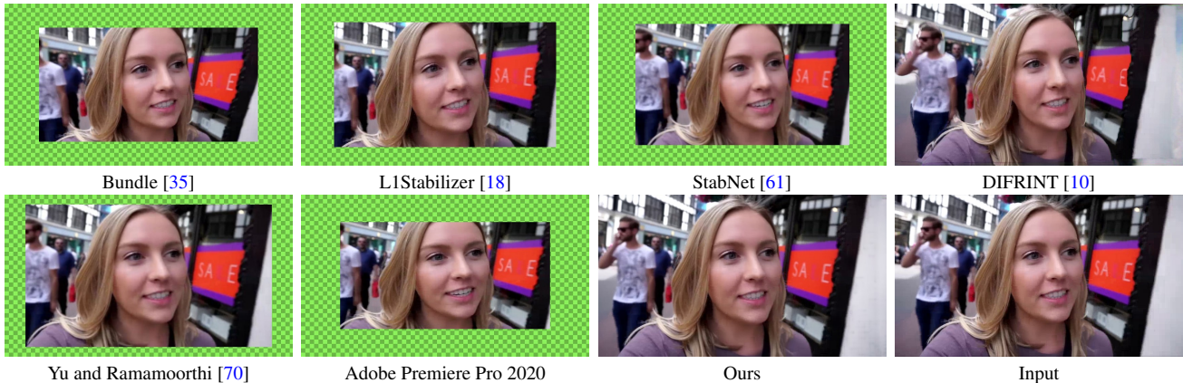
Figure 5: Visual comparison to state-of-the-art methods. Our proposed fusion approach does not suffer from aggressive cropping of frame borders and renders stabilized frames with significantly fewer artifacts than DIFRINT [10]. We refer the readers to our supplementary material for extensive video comparisons with prior representative methods.
