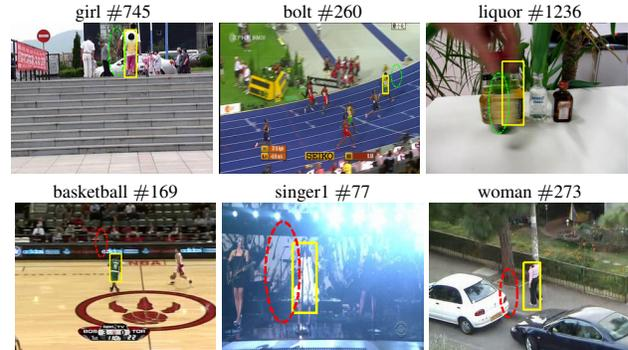
Figure 5. Tracking results with comparisons to color-based trackers. The results by the MS tracker, PF method and our algorithm are represented by red ellipse, green ellipse and yellow rectangles. It is evident that our tracker is able to handle cluttered background (*girl* and *basketball* sequences), drastic movement (*bolt* sequence), heavy occlusion (*liquor* and *woman* sequences) and lighting condition change (*singer1* sequence).
