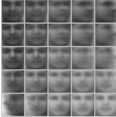
Figure 9: Prototype of each face class using Kohonen’s SOM by Yang, Ahuja and Kriegman [175]. Each prototype corresponds to the center of a cluster.
