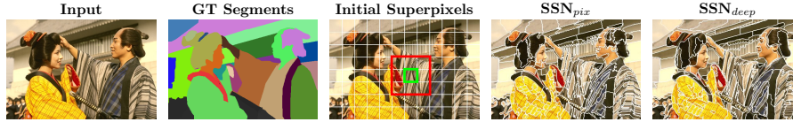
Fig. 2: From initial grid to learned superpixels. An example visual result from BSDS500 dataset showing the initial superpixel grid and the superpixels obtained with SSN_{pix} and SSN_{deep} . To compute the pixel-superpixel associations for every pixel in the green box, only the surrounding superpixels in the red box are considered.
