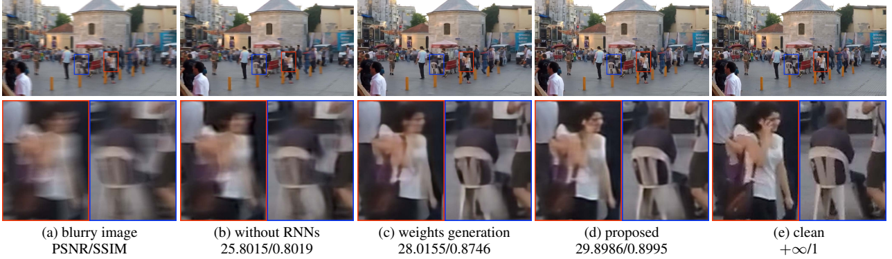
Figure 9. Visual results for the ablation study on the dynamic scene dataset [21]. The proposed method generates clearer images with higher PSNR and SSIM values relative to the networks with only CNNs. Refer to the text for details.
