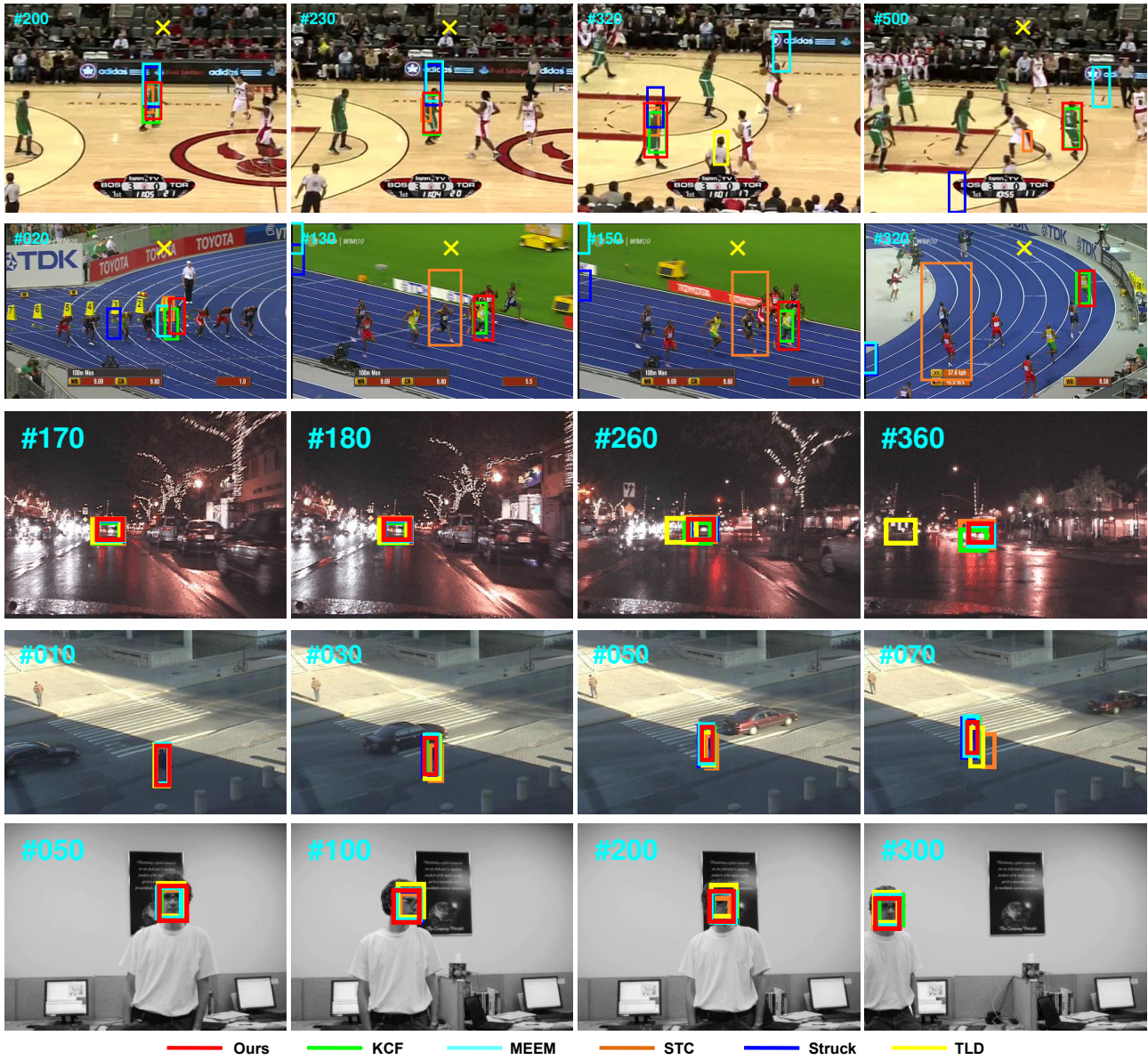
Figure 2. Tracking results of our proposed algorithm, KCF, STC, and TLD methods on six challenging sequences (from top to down are Basketball , Bolt , CarDark , Crossing , and David2 , respectively). A case of tracking failure is denoted by \times .
