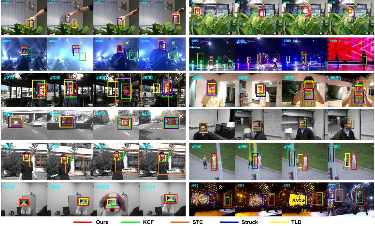
Figure 7. Tracking results of our LCT algorithm, KCF [11], STC [28], Struck [9] and TLD [14] methods on twelve challenging sequences (from left to right and top to down are Coke , Tiger2 , Shaking , Skating1 , Trellis , David , Car4 , Fleetface , Jumping , Jogging-2 , Dog1 , and Singer2 , respectively).
