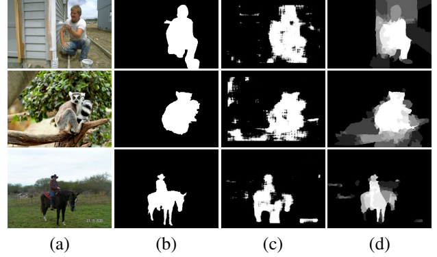
Figure 4. Saliency maps by local estimation. (a) Source images. (b) Ground truth. (c) Local saliency maps predicted by DNN-L . (d) Local saliency maps after refinement.
