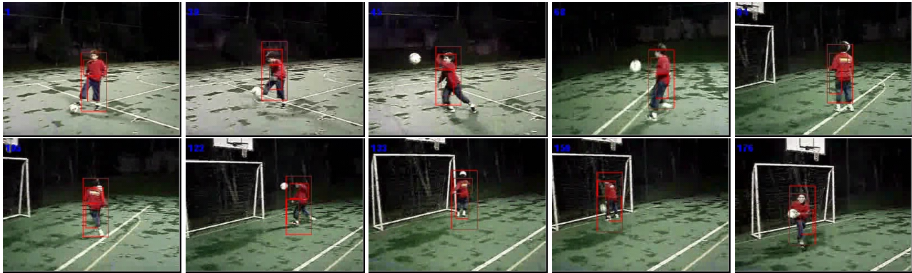
Figure 9. Tracking results using the proposed algorithm. Shape and appearance variations are substantial in this sequence.
