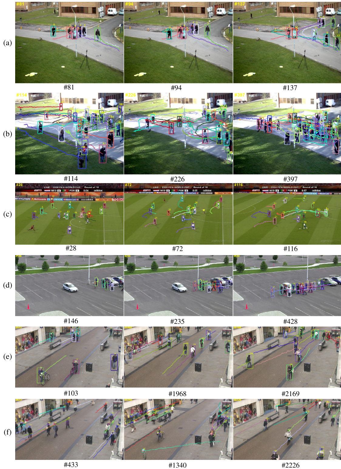
Fig. 8. Sample tracking results for five sequences, the arrangement from top to bottom as (a) and (b) PETS09-S2L1 , and PETS09-S2L2 , respectively, (c) Soccer sequence, (d) UCF-PL sequence, (e) Town Center dataset (body), and (f) Town Center dataset (head).
