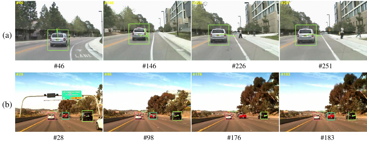
Fig. 9. Sample tracking results for LISA 2010 dataset, where (a) and (b) correspond to Urban and Sunny sequences, respectively.
