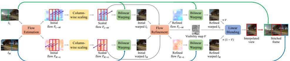
**Figure 5: Pushroom interpolation layer.** A straightforward implementation of the pushroom interpolation layer requires to generate all the intermediate flows and the intermediate views, which is time-consuming when the number of interpolated views  $K$  is large. Therefore, we develop a fast pushroom interpolation layer by a column-wise scaling on optical flows, which only requires to generate one interpolated image for any given  $K$ .
