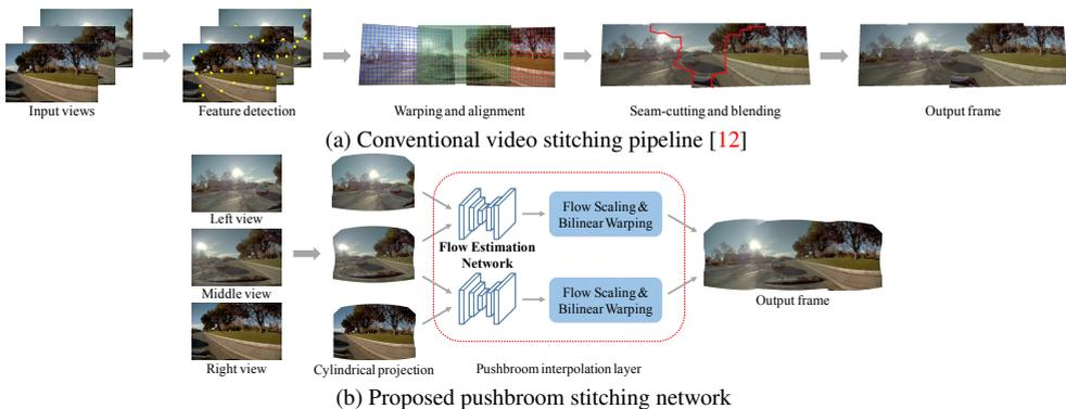
**Figure 2: Algorithm overview.** (a) Conventional video stitching algorithms [12] use spatio-temporal local mesh warping and 3D graph cut to align the entire video, which are often sensitive to scene content and computationally expensive. (b) The proposed pushbroom stitching network adopts a pushbroom interpolation layer to gradually align the input views, and outperforms prior work and commercial software.
