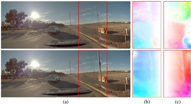
Figure 7: **Visualization of the stitched frames and flows.** We show the stitched frames (a), forward flows (b), and backward flows (c) from the pushbroom interpolation layer before (top) and after (bottom) fine-tuning the proposed model. The fine-tuned model generates smooth flow fields to warp the input views and preserve the content (e.g., the pole on the right) well.
