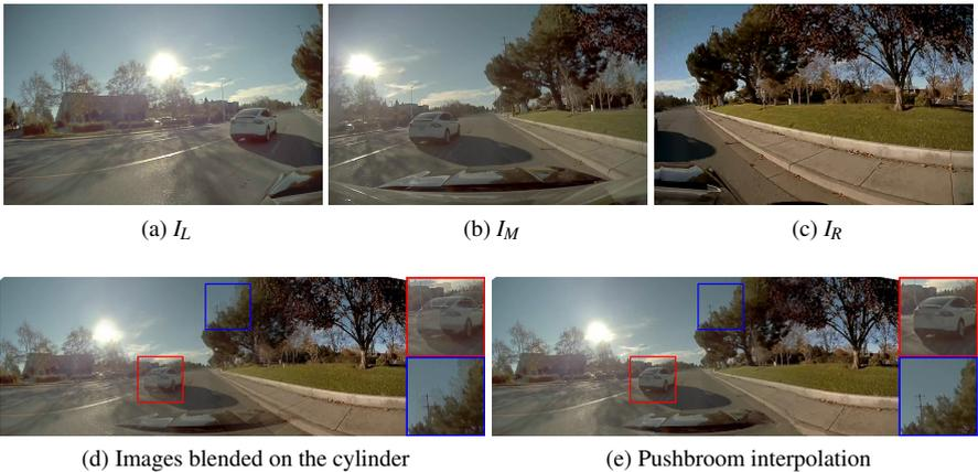
**Figure 4: Example of input and stitched views.** Simply projecting the input views  $I_L$ ,  $I_M$ , and  $I_R$  onto the output cylinder causes artifacts due to the parallax and scene depth variation (d). Our pushroom interpolation method effectively stitches the views and does not produce ghosting artifacts (e).
