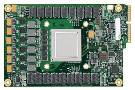
**Figure 3.** TPU Printed Circuit Board. It can be inserted in the slot for an SATA disk in a server, but the card uses PCIe Gen3 x16.
