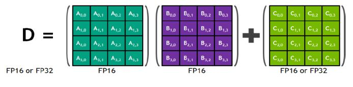
Figure 8. Tensor Core 4x4 Matrix Multiply and Accumulate
