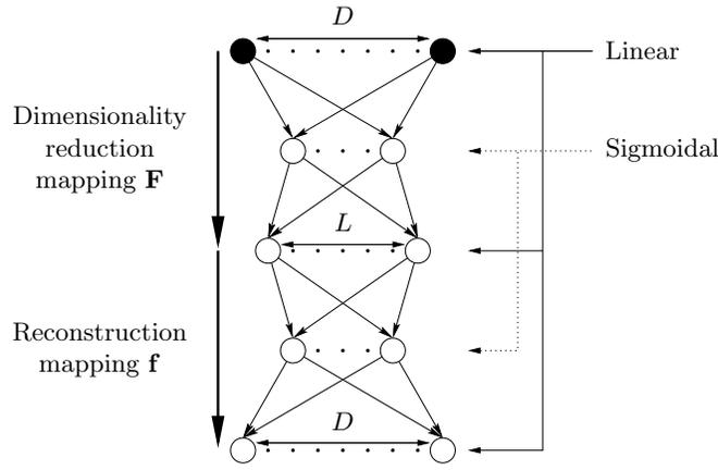
Figure 4.10: Nonlinear autoassociator, implemented as a four-layer nonlinear perceptron where  $L < D$  and  $\mathbf{t}^* \stackrel{\text{def}}{=} \mathbf{f}(\mathbf{F}(\mathbf{t}))$ .
