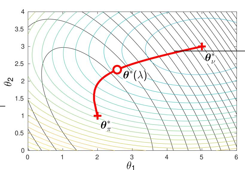
$\theta^*(p)$  is an optimal classifier (minimizing  $\nu$ ) with an FP rate of at most *p*. The infeasible set is in pink. The contours of  $\nu$  and  $\pi$  are in color and black, respectively.
