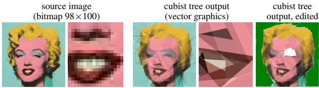
Fig. 7. Plots 1–2: source image and zoomed-in region (mouth and nose). The original pixels are clearly visible. Plots 3–4: cubist tree output and zoomed-in region in the same area. The (infinite-resolution) poxels are visible. Plot 5: cubist tree output edited with Inkscape to color some of the polygons in the background in green, and to move away some of the polygons in one eye to the right side.
