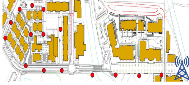
Fig. 10. Location B Mesh topology - nodes populated at the gray region.
