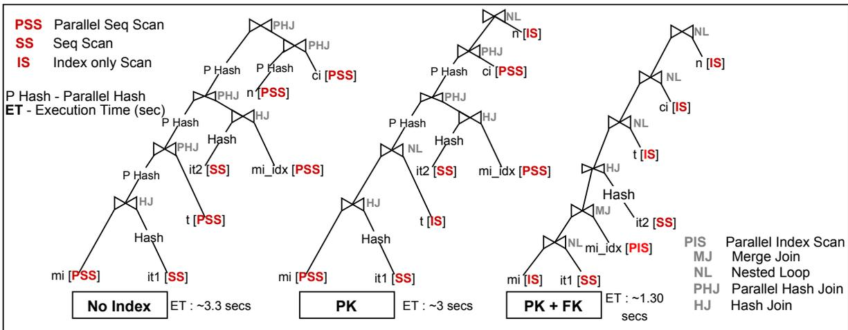
Figure 6: Pessimistic: Physical operators in different index configurations.
