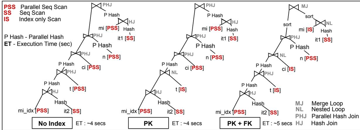
Figure 4: Simplicity: Physical operators in different index configurations.
