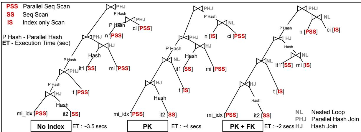
Figure 7: Simpli<sup>2</sup>: Physical operators in different index configurations.
