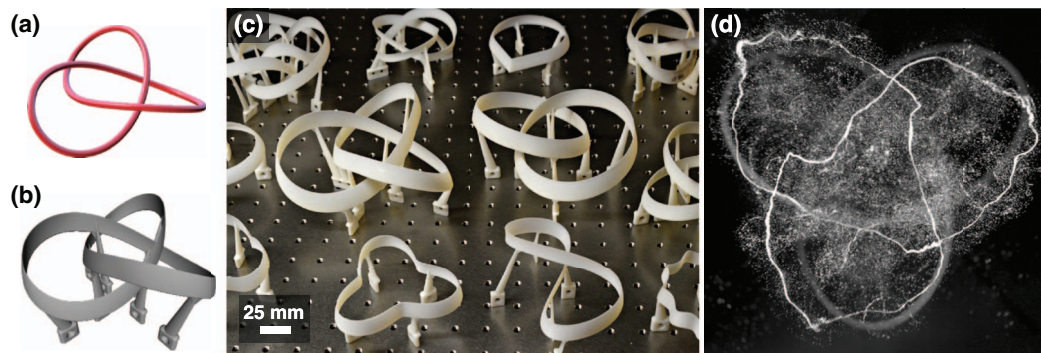
FIG. 1. The process for designing a vortex of a desired shape. (a) A 3D path of the desired vortex shape is created, and (b) converted into a 3D model of a hydrofoil whose trailing edge traces this shape. Struts which connect the hydrofoil to the acceleration frame are also added. (c) The 3D model is printed with a rapid prototyping machine. Examples of hydrofoils are shown in a number of geometries and topologies. (d) The hydrofoil is accelerated in a tank of water, generating a vortex which is traced with buoyant micro-bubbles. The hydrofoil which created this vortex knot is faintly visible in the background. [URL: http://dx.doi.org/10.1063/1.4893590.1 ]
