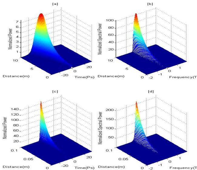
**Fig. 2** Similariton evolution in a 10-m long GGF (a) time domain (b) frequency domain. Similariton evolution in a 10-cm long erbium fiber amplifier (c) time domain (d) frequency domain.
