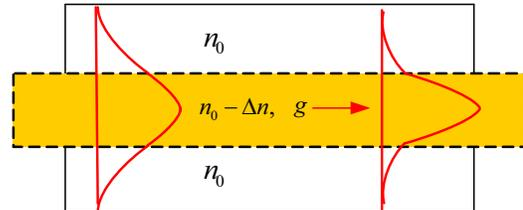
Fig. 1 Gain guiding plus index anti-guiding, with a negative index step:  $-\Delta n$  in the core
