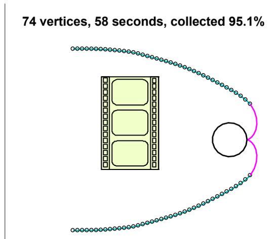
Video 2. [cylindrical\_absorber\_movie.mp4]. A concentrator for a cylindrical receiver (black circle). The section (in magenta) to the right of the receiver is kept fixed. The optimization algorithm is applied to the top segment and reaches 95% collection efficiency using 74 vertices. <http://dx.doi.org/10.1117/12.2503895.2>
