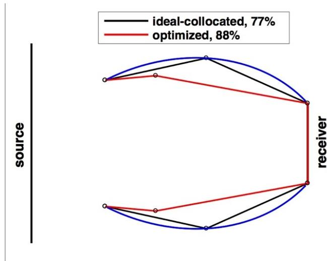
Figure 1. The optimized concentrator design using a single-vertex polygon (red) yields 88% collection. In comparison, the ideal-collocation design (black), which is obtained by placing the vertex at the center point of the ideal shape (blue), yields 77% collection.
