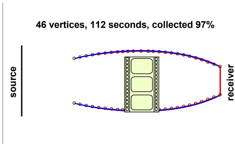
Video 1. [planar\_absorber\_movie.mp4]. A concentrator for a planar receiver (line segment on the right side). The optimization algorithm converges to the ideal shape (blue curves), reaching 97% collection efficiency using 46 vertices. The wall-clock runtime (seconds) is shown. <http://dx.doi.org/10.1117/12.2503895.1>
